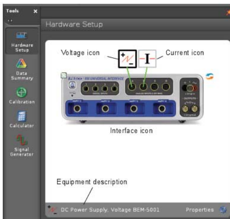
Figure: Hardware Setup Window
