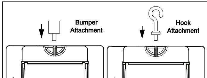
The Magnetic Bumper has a metal post that fits in the small hole to the side of the threaded hole in the front end of the Smart Cart. The post ensures that the Magnetic Bumper is mounted in the correct orientation.
