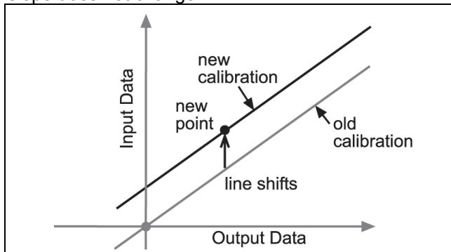
Offset calibration is usually used to make one sensor agree with another sensor. Due to normal variation among probes, a second probe might read consistently higher than the first probe. Normally this difference would be insignificant; however, an offset calibration can be used to bring the sensors into closer alignment.
