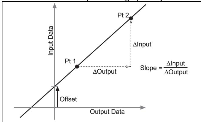
Two points, Pt 1 and Pt 2, define the line. In the two-point calibration procedure, each point is reset by associating a known standard value (for instance, the temperature of ice water) with a raw input measurement that the sensor sends out when it is in that standard. In a one-point calibration, only one of the points is reset by the user.
